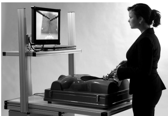
Figure 1. ProMIS Augmented Reality Laparoscopic simulator (Haptica, Dublin, Ireland), with the needle-holders (Karl Storz, Tutlingen, Germany) and versaport trocars 5mm (Tyco Auto Suture, New Haven, USA).
