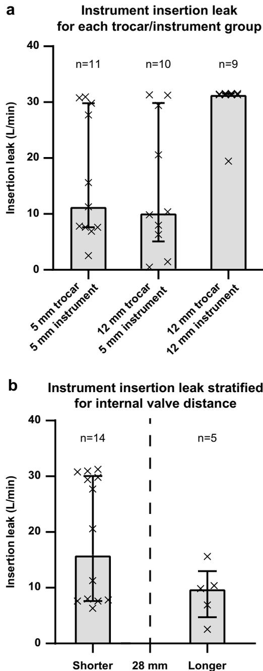
**Fig. 5** **a** Leak during instrument insertion trocars grouped per trocar size and used instrument size, median and inter-quartile range per group. **b** The effect of valve distance compared to the tool tip length of the surgical instrument, in this case longer or shorter than 28 mm. The height of the boxes is the median value, the whiskers represent the inter-quartile range and the crosses are each individual trocar
