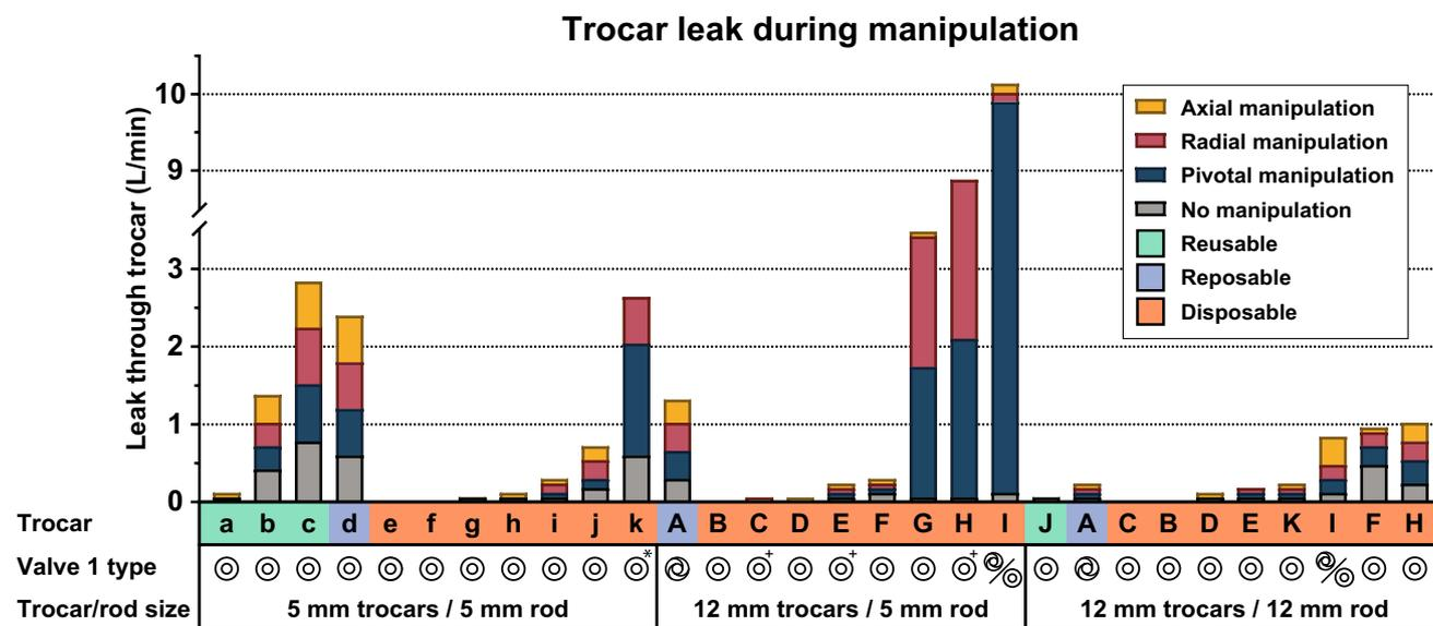
Fig. 4 Leak through trocar caused by different manipulations with a solid shaft. The symbols below the bars indicate the type of valve 1 that was used on each trocar. The shaft size, number of valves and
