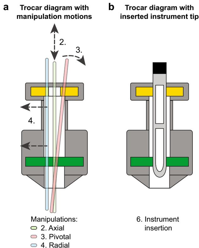
**Fig. 2** **a** Manipulations of the rod within the trocar, in axial (2), pivotal (3) and radial (4) directions. Axial manipulation oscillations are performed with a 5 cm amplitude. During the pivotal and radial manipulation the rod is maximally displaced. **b** During the instrument insertion test, a grasper with a fenestrated structure was inserted into the trocar and kept in contact with both valves to allow for an open passage of gas
